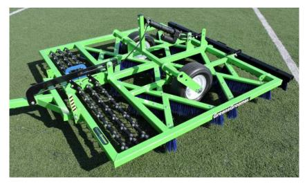
design are the precise brush dimensions and angles. This allows grooming in four directions, standing up turf fibers and leveling infill material. The integrated rake simplifies equipment requirements and gives the facility flexibility for on-demand raking without equipment change-over.
