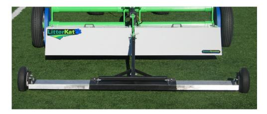
The tow-behind Sports Field Magnet is a necessary component for proper turf maintenance. The pickup of unwanted ferrous objects is handled by a powerful, industrial magnet that is capable of pulling objects deep from within the turf.
