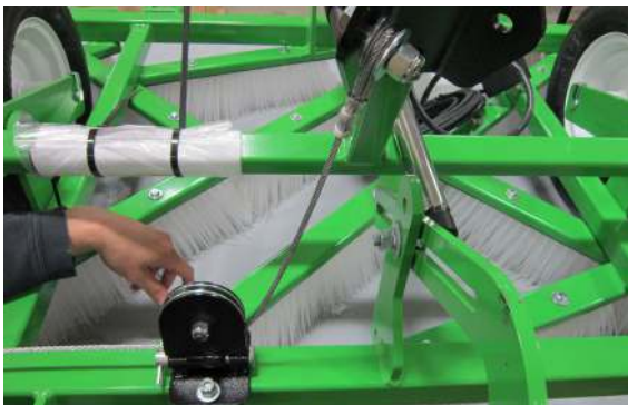
Attach the cable sheave bracket to the frame of the Groomer. The sheave bracket should be placed 26-1/2 inches from the outside of the GreensGroomer frame.
