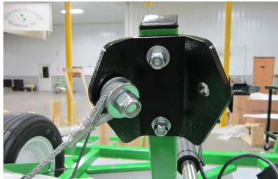
Attach the cable bracket to the upright arm of the wheel assembly using the longer bolts included to make up for the added thickness. Attach one end of the cable to the bracket.
