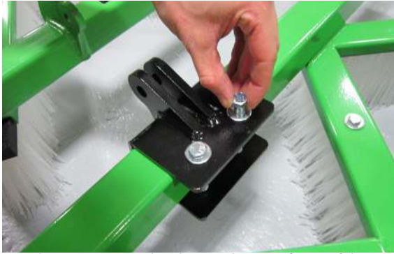
Attach extension wing brackets to the main frame of the Groomer. Do not tighten.
