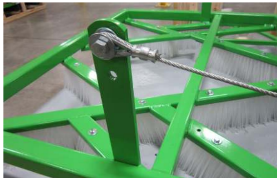
Attach the loose end of the cable to the upright arm of each wing.
